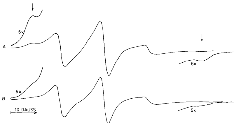
Fig. 1. ESR spectra of spin labeled GluDH. Conditions: Protein 13 mg/ml. Buffer 0.05 M Tris–0.1 M NaCl pH 7.4. The labeling reaction was carried out without additions (A) and in the presence of 3.1 mM NADH and 1.8 mM GTP (B). The arrows indicate the positions of the outer peaks of the immobilized spectrum. The spectra were recorded using a power of 20 mW and a modulation amplitude of 0.8 G.
